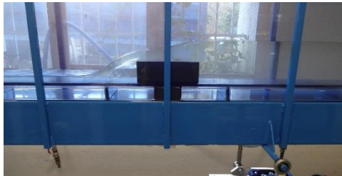
Weir thick threshold
